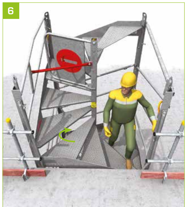
- Make sure that the tethers are fitted before detaching the slings. - Tilt the guardrails to create the exit at the desired level.
